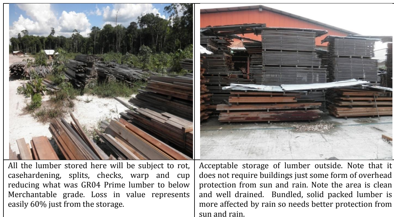
Figure 24: Proper and improper storage of lumber
